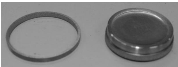
Fig. 5: Coated test sample after testing (right) showing coating ring sheared from circumference (left)
